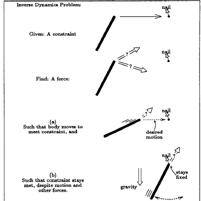
Figure 6: The inverse dynamics problem for dynamic constraints.
